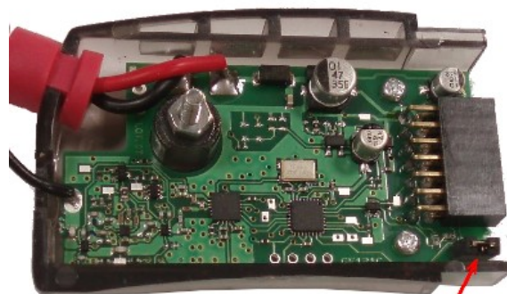
Jumper: remove for SCP 1.1 and 2 leave for SCP 1.0
