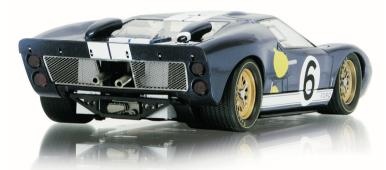
Visually, the MKII was little different from the standard GT40s. The car was very stable at high speeds after the lifting habit of the early models was solved. The MKII used the 7.0 liter (427ci) engine derived from the Ford Galaxie, with aluminum head; the power was 485 hp at 6300 rpm, and the car was able to reach a maximum speed of 330 km/h. The chassis was a steel semimonocoque, with a glass fiber body. The disc brakes were ventilated on the four wheels.
