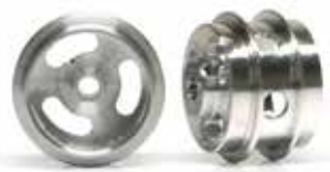
W15810215AH ex PA49-Alh Al Ø15.8 x 10.2 x 1.5mm wheels, double shoulder holed channel, M2 grub - 1.2g (2x)
