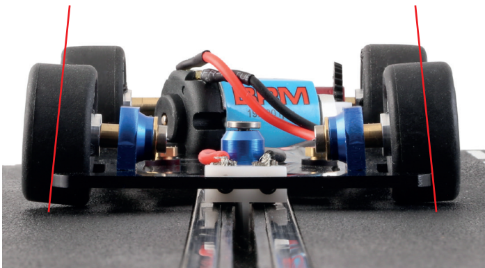
Front: Independent steel axle "CAMBER"
