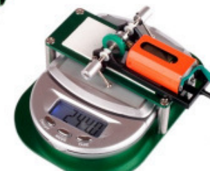
Ref. 60101 Banco Motor Miniscale Torque Magnetic power
