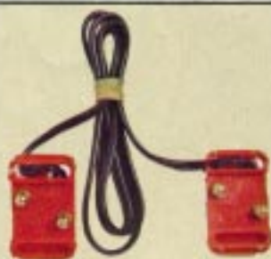
C.252 Power Boost Connectors (Set of 2) For use on large layouts to avoid a voltage drop on the parts of the layout that are some distance away from the Hand Throttle track connections. They plug into any Full Straight, one end near the Hand Throttles and the other end on the far side of the layout. Care must be taken to connect not only the same lane but also the same rail, otherwise a short circuit will occur.
