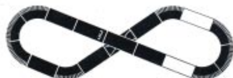
2nd extension — add 2xC.160 Straight 'D' Area approx. 8'6" x 3'0" (260cm x 92cm)
