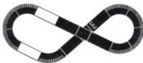
1st extension — add 2x C.160 Straight 'D' Area approx. 7'0" x 3'0" (213cm x 92cm)
