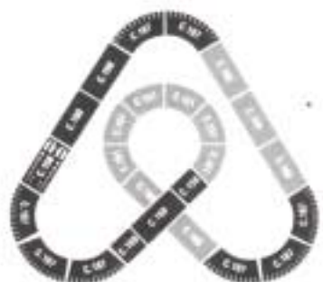
Banked Figure 8 Circuit Suggested Extension 2 Requires 6 x C.151 5 x C.160 Approximate size 5'9" x 5'6" 175 x 167 cms.
