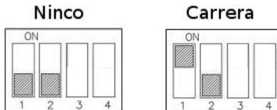
Use this DIP switch configuration *only* if you want to leave the original electronics in place, alongside oXigen's.
