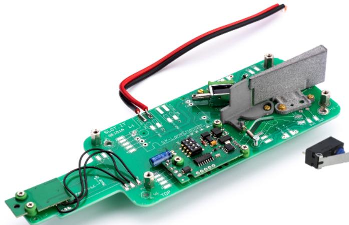
The flipper maximum operating time is 300ms: it is shortened if a chasing car is detected and said car doesn't request a lane change, or if the optional switch is activated.
