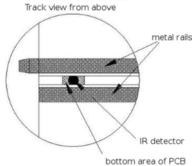
Beware: if you look at the bottom side of the track, the component side of the sensor board must be visible.
