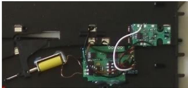
For *Ninco* track, the opening is already present; for *Carrera* track, drill a hole in the bottom of the slot. Make sure the IR detector is properly placed – you must be able to see it from above.
