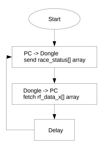
The 'delay' value is strictly connected to the speed of the PC speed and its tasks' load, and this in turn may affect the speed of the RMS. Note that each controller sends its data back to the dongle with a 600ms cycle time (i.e. every 600 ms).
