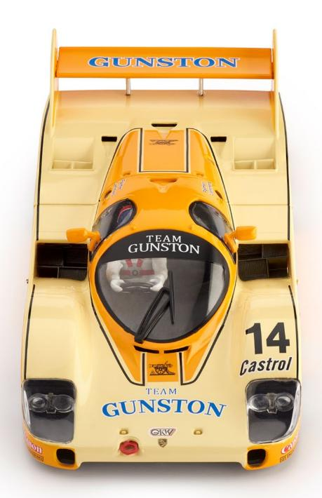
The Porsche 956 and later 962 models could be assembled with two different rear wing configurations: "low downforce", used mostly in Le Mans where the 6.5 km Hunaudières straight required a very low drag at the expense of downforce, and "high downforce", for twistier circuits. Regardless of the configuration, Porsche 956 and 962 cars were the cars to beat in any Group C competition in the early 80's.
