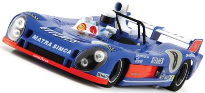
The version used in '74 for Le Mans was the 'MS 73', with a maximum torque of 320 Nm at 8400 rpm , reaching a maximum power of 450 HP at 10500 rpm. On the Mulsanne straight the car could top 320 kph.
