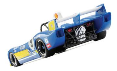
The version used in '74 for Le Mans was the 'MS 73', with a maximum torque of 320 Nm at 8400 rpm, reaching a maximum power of 450 HP at 10500 rpm.
