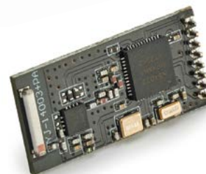
SCP301b oXigen RF power amplifier for oXigen system
