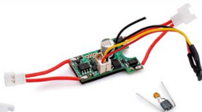
0201b2 oXigen chip in-car controller (type B)
