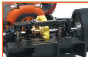
CH47b Universal spring suspension kit
