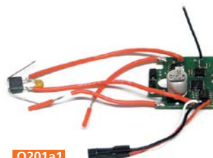
O201a1 oXigen chip In-car controller (type A)
