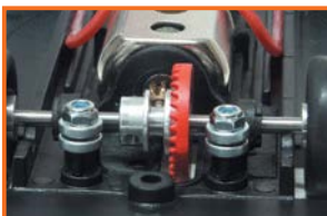
CH09 Magnetic suspension kit
